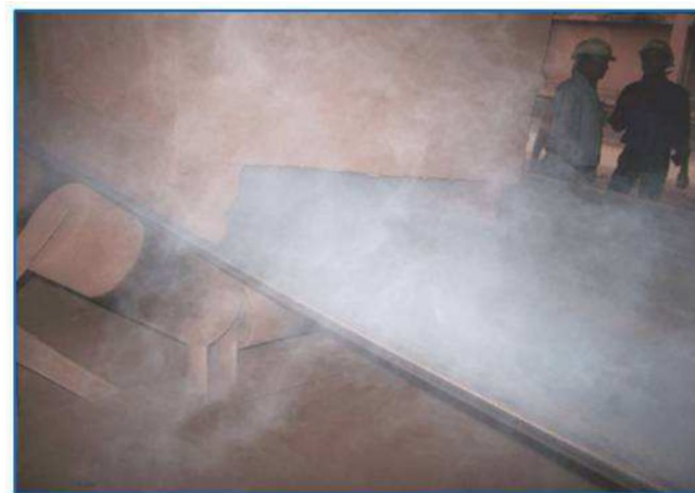
Dry Fog Dust Suppression System at Conveyors
