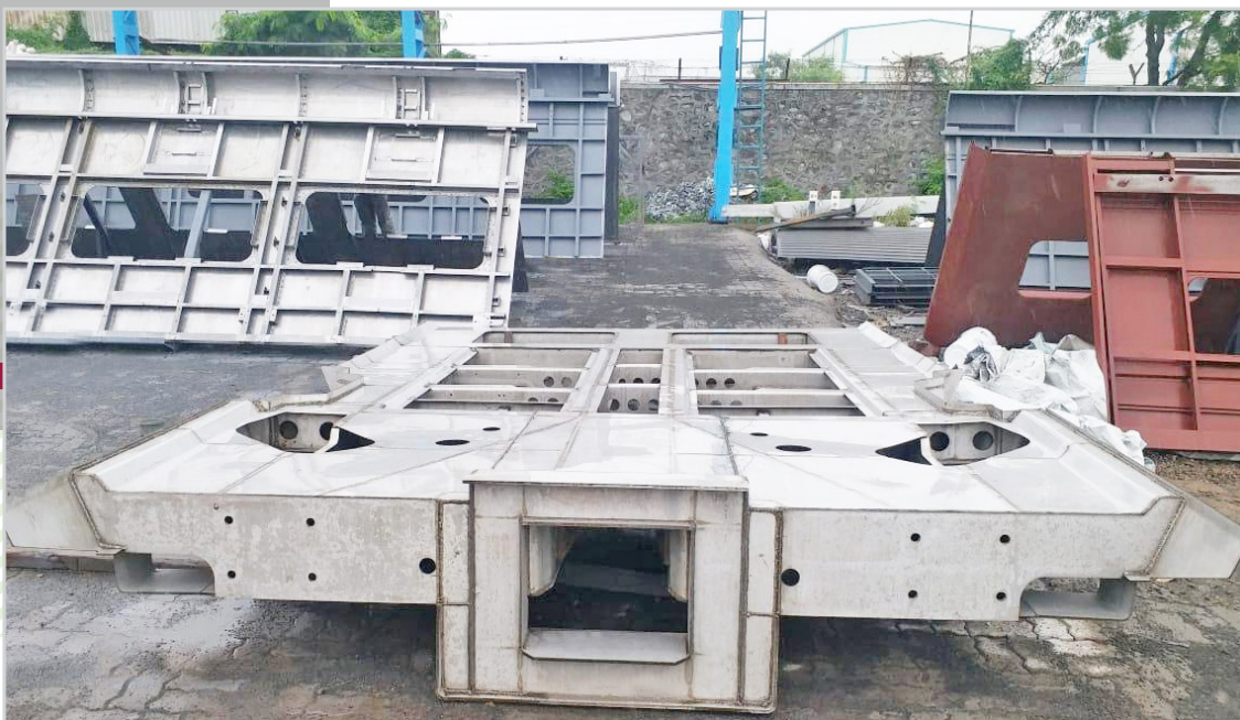
Stainless steel underframe in SS 201LN grade.
