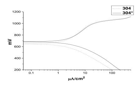
Test Solution: 50% Nitric Acid at 25degC
