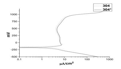
Test Solution: 50% Formic acid at 25degC
